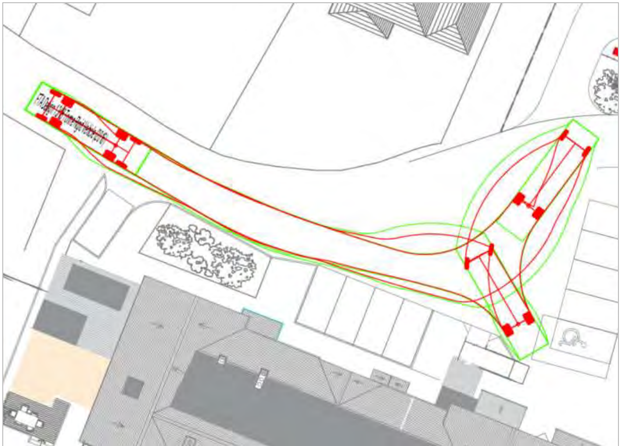
Figure 4.8: 10m rigid vehicle turning
