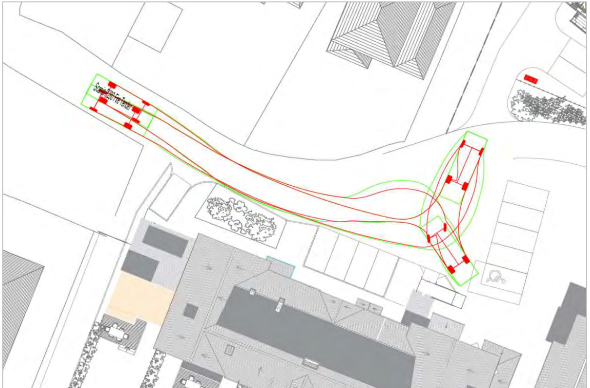
Figure 4.6: Scania P280 fire tender turning in centre of site
