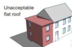
Two storey side extensions should be subordinate in scale to the original house.
