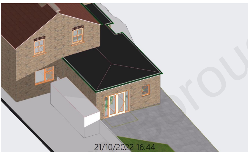
4 March/October equinox 16:45 GMT Shadow remains until sunset, with existing neighbouring outbuilding over-shadowing window too
