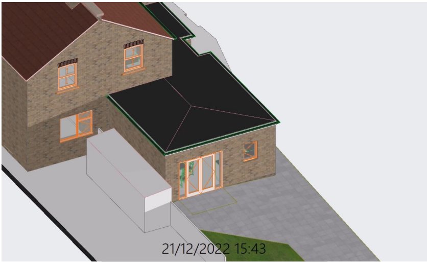
2 Winter solstice sunset 15:45 GMT Shadow from proposed extension remains across neighbouring window until sunset at 3.45pm
