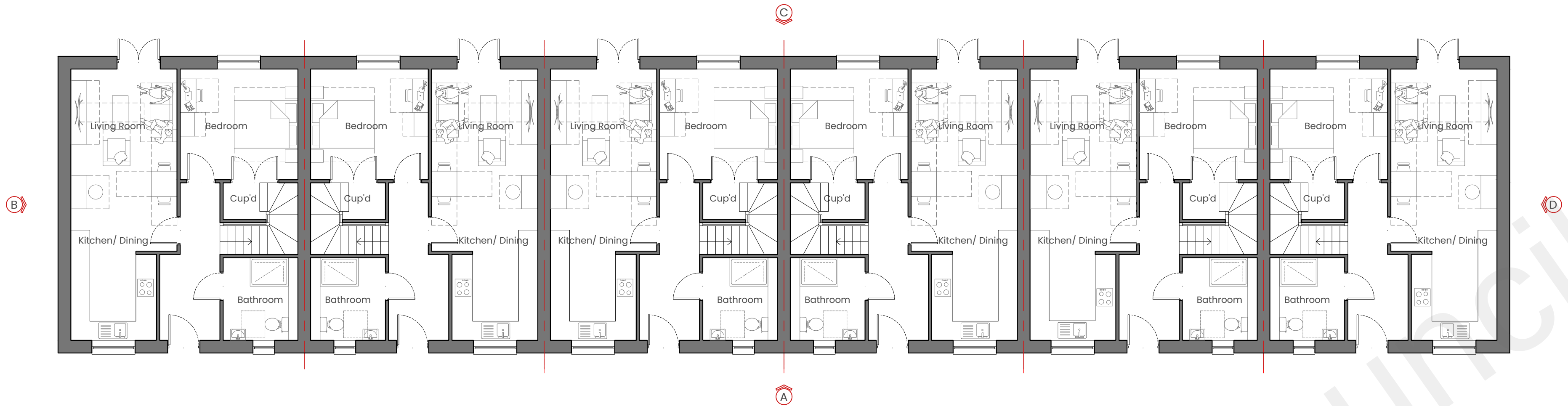
Ground Floor Plan As Proposed GIFA= 60.85m 2 Per Unit
