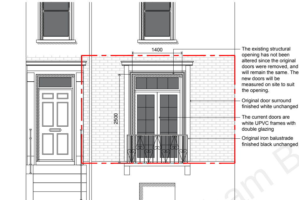
01 | 1:50 | EXISTING FRONT ELEVATION
