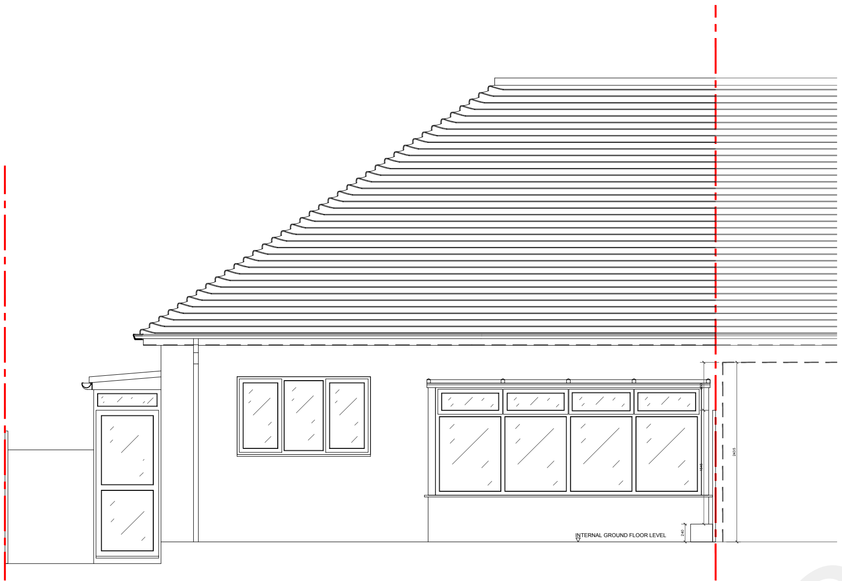
EXISTING REAR ELEVATION SCALE 1:50 @ A1 / 1:100 @ A3
