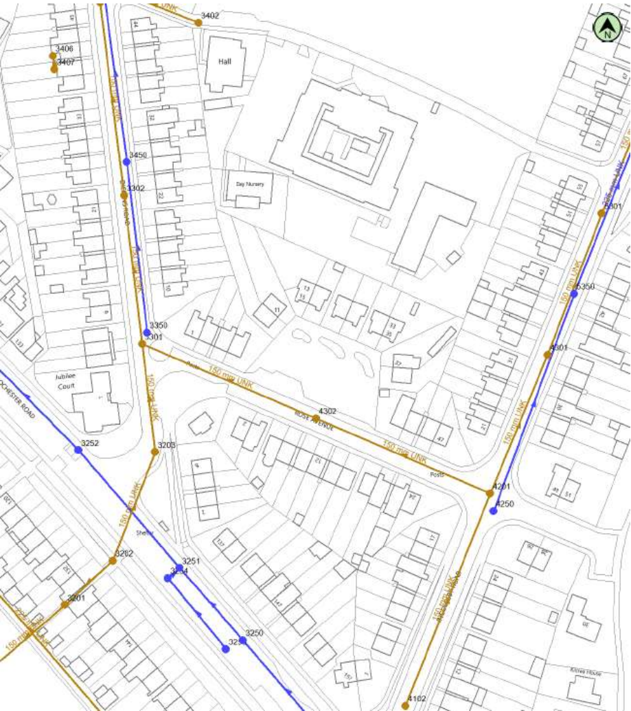
Figure 5 - Extract of sewer records
