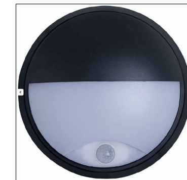
IP54 LED Luceco Eco Bulkhead Eyelid Wall Light with PIR 4000k Warm White colour temp. 10W & 400 lumens.
