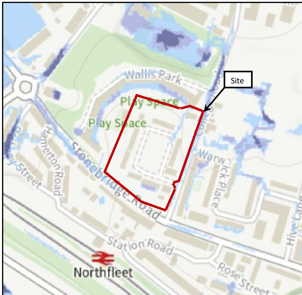
Figure 4.1 – Environment Agency Indicative Surface Water Flood Mapping
