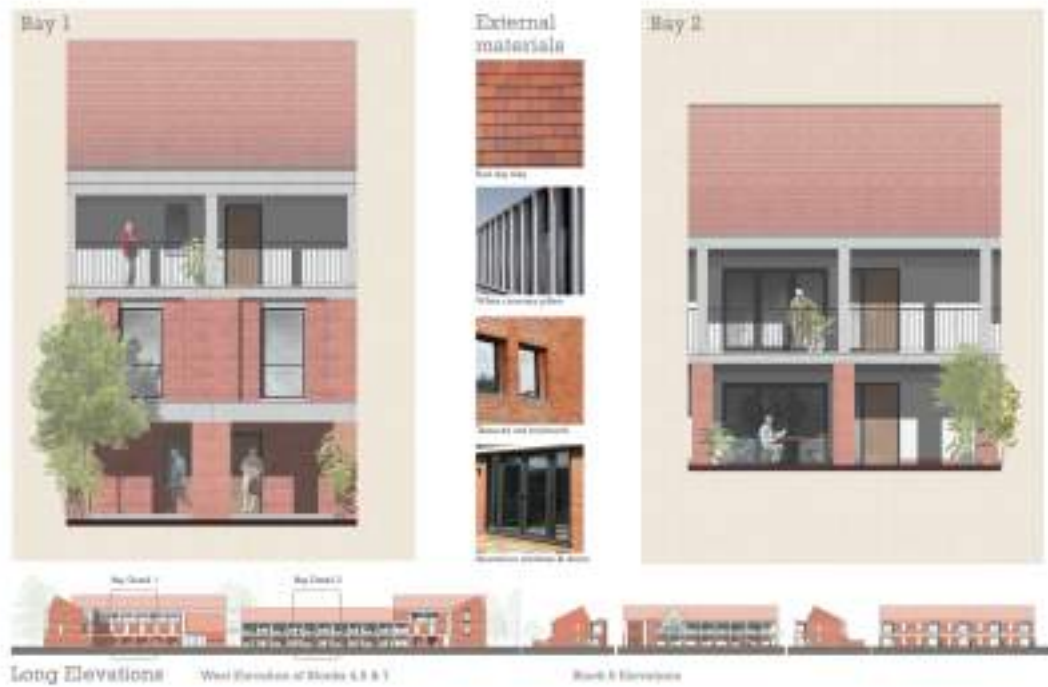
Board 5: Detail elevations and materiality studies.
