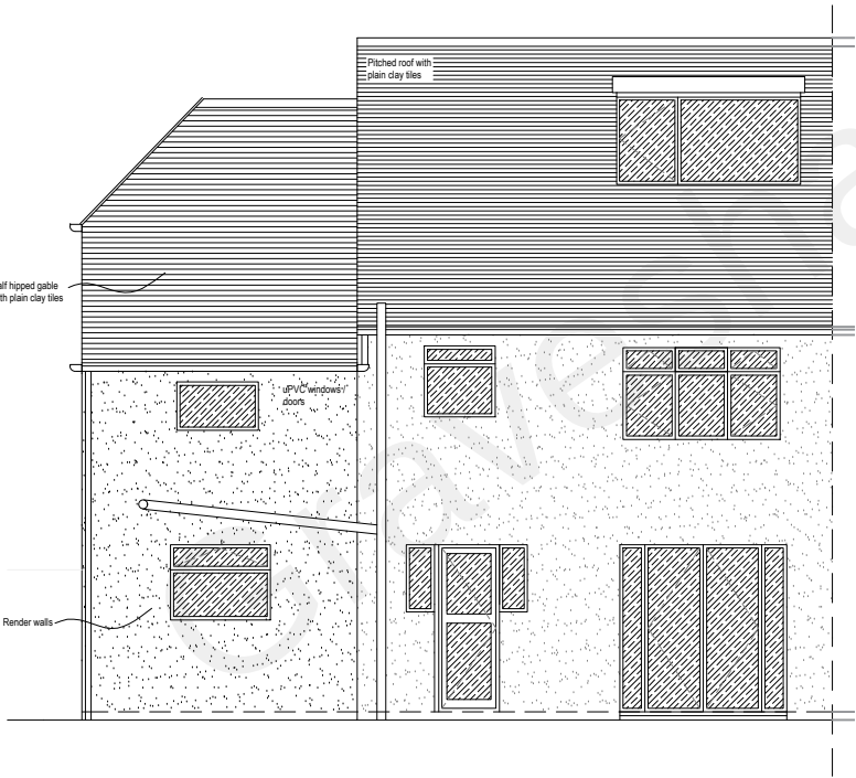
EXISTING REAR ELEVATION
