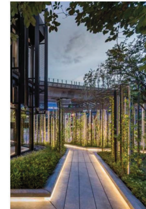
Light fitting recessed in planters to wash light on circulation routes and public square
