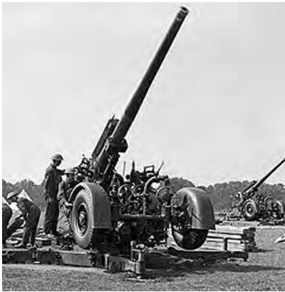
British H93 Gun in Hyde Park 1941. The 3.7" anti-aircraft gun could propel High Explosive and Incendiary shells up to 59,000 feet, higher than the German bomber aircraft could fly.
