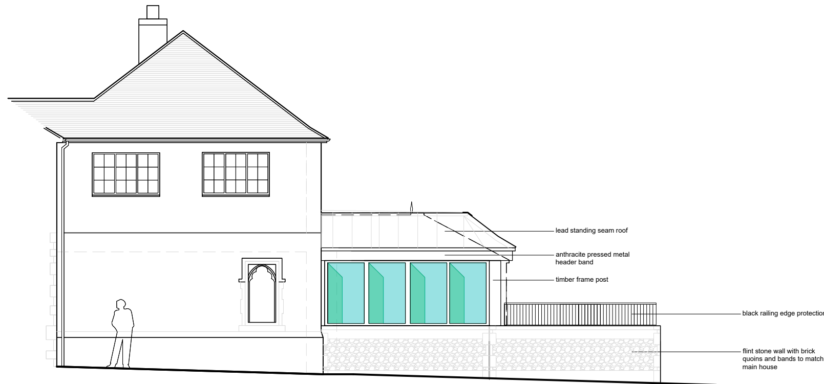
PART EAST ELEVATION vegetation omitted for clarity
