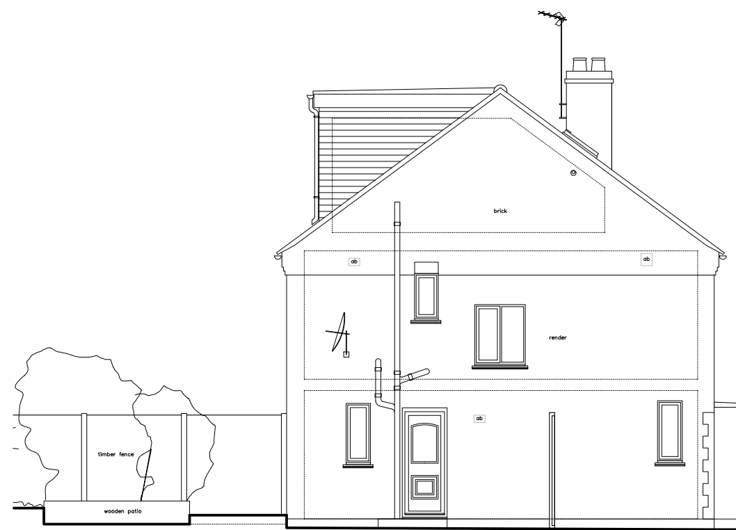
side elevation 1:100 (as seen from no 34)
