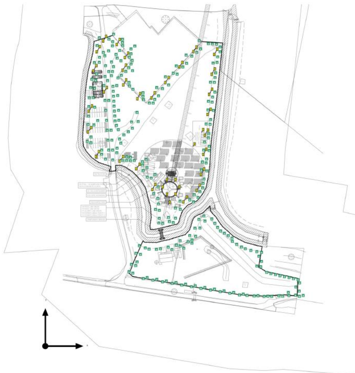
Figure 11 Indicative lighting points within site boundary – Note that the figure is an indicative scheme of the lighting array. The lighting will be installed on the internal face of the hoarding, directed away from the watercourse, and designed as per condition 11.
