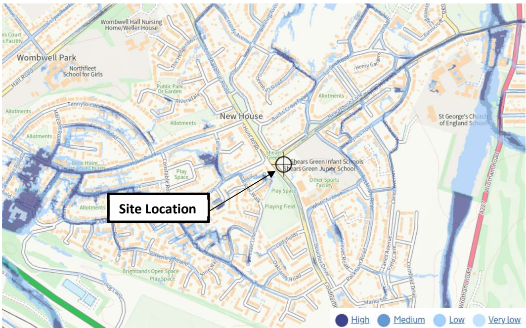
Figure 5 - Flooding from Surface Water
