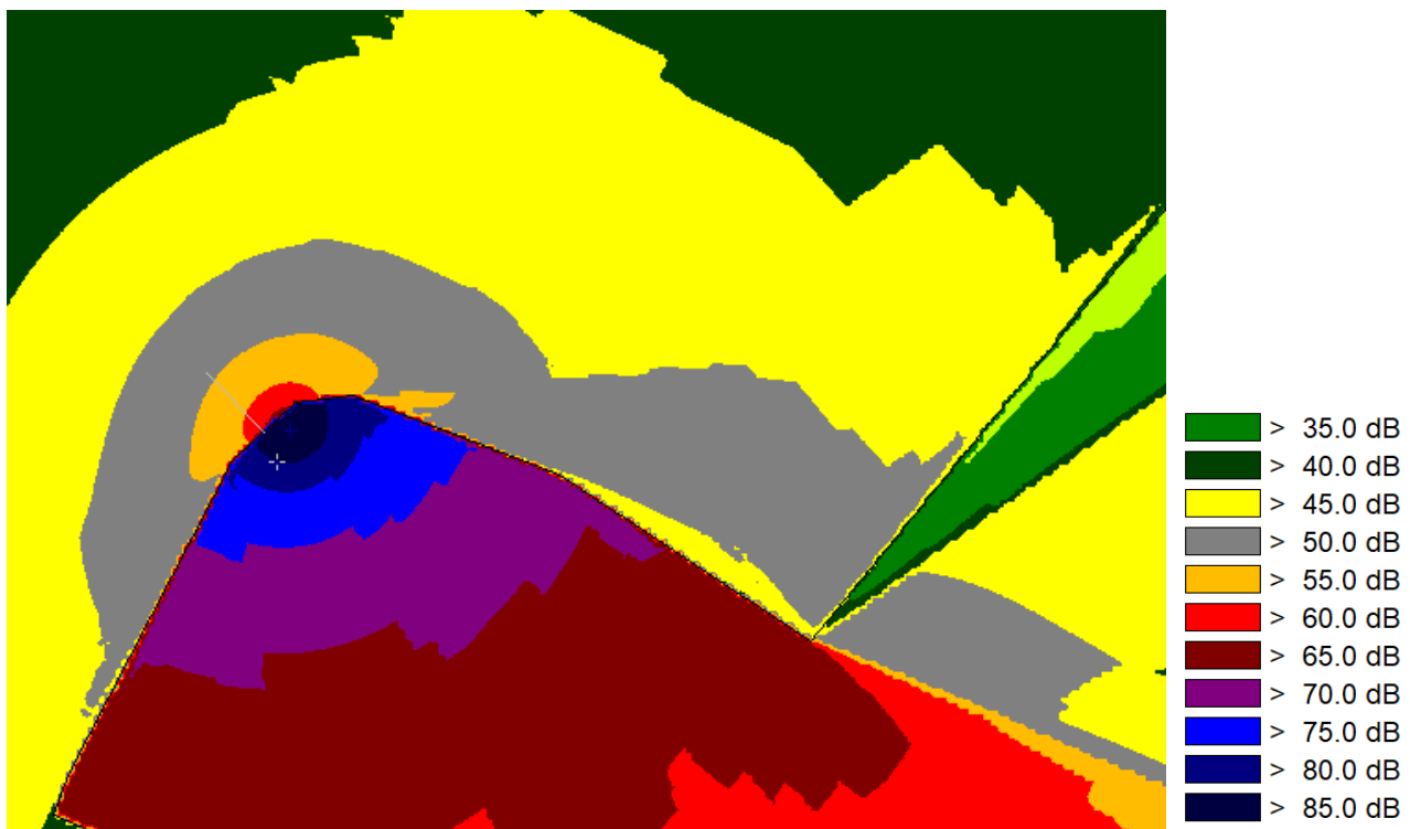
Figure 13: Noise levels with perimeter barrier installed
