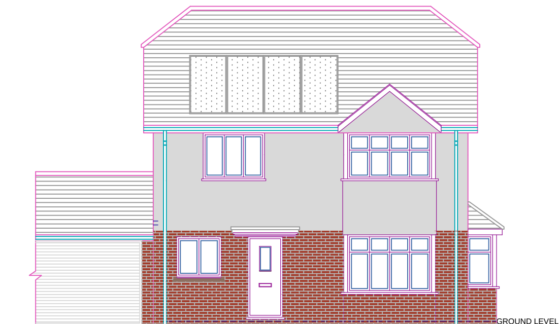
PRE EXISTING FRONT ELEVATION
