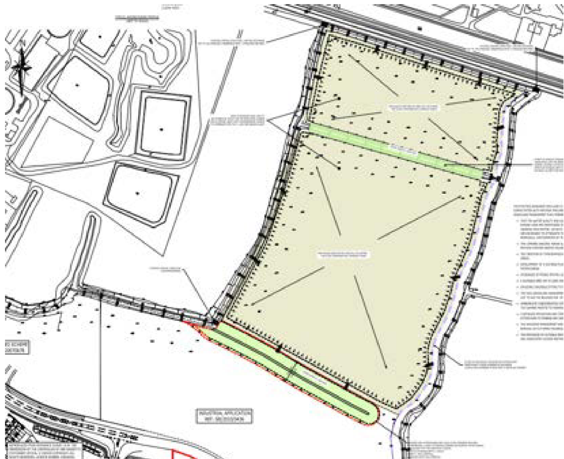
Figure 3 - Watercourse provision and flood levee excavation work.
