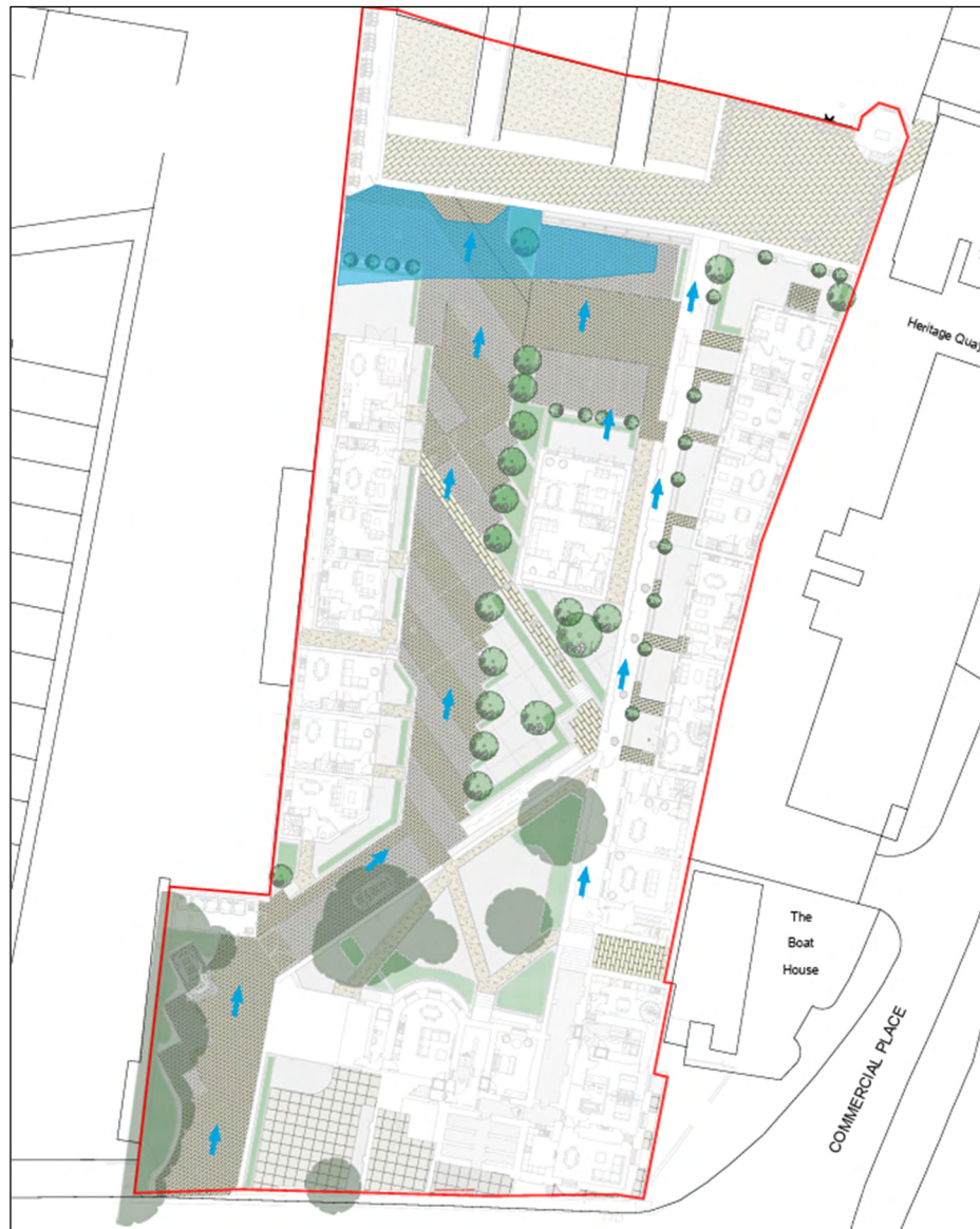
Figure 1 – Anticipated flow routes during an exceedance or blockage event.
