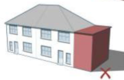
Incorrect extensions in terms of position, scale and roofline.
