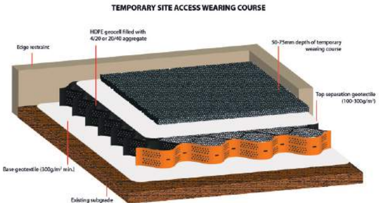
Figure 5: A geocell surface used during construction needs to be protected by a temporary wearing course and an upper geotextile is required to prevent mud from migrating down into the infill [image courtesy of Core LP].
