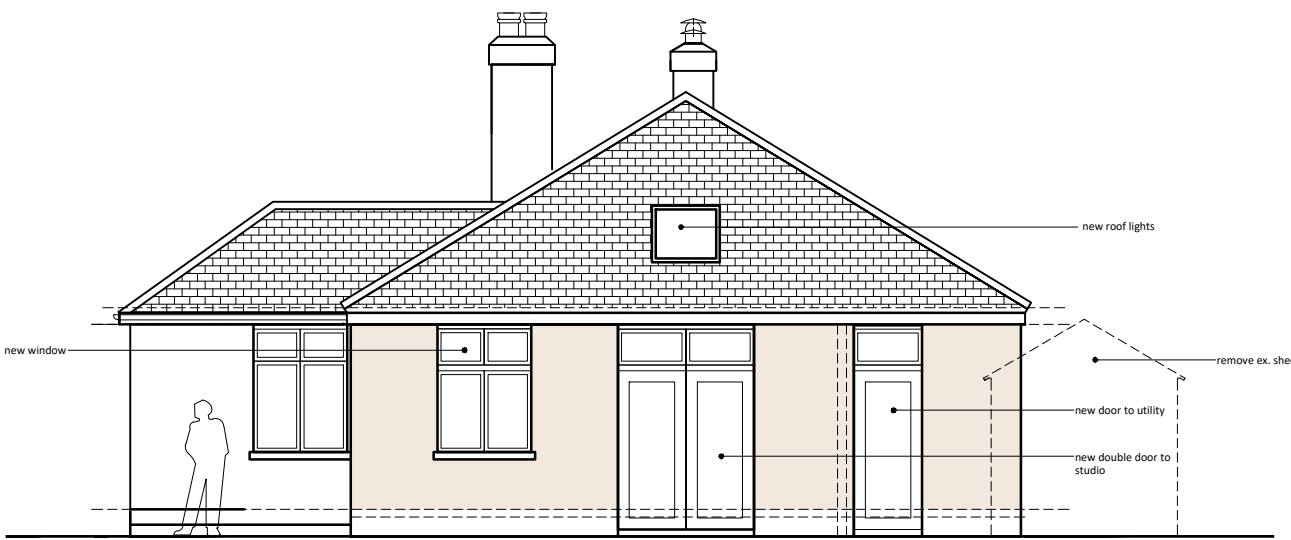
PROPOSED NW ELEVATION
