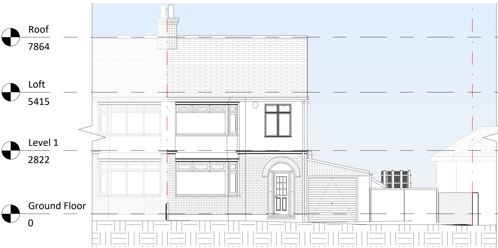
4 Existing Front Elevation 1 : 100
