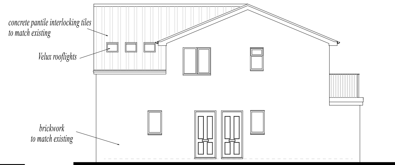
SIDE ELEVATION (NORTH)
