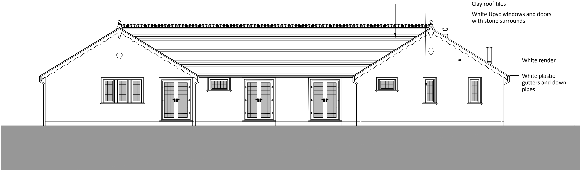
Existing West Elevation 1:100
