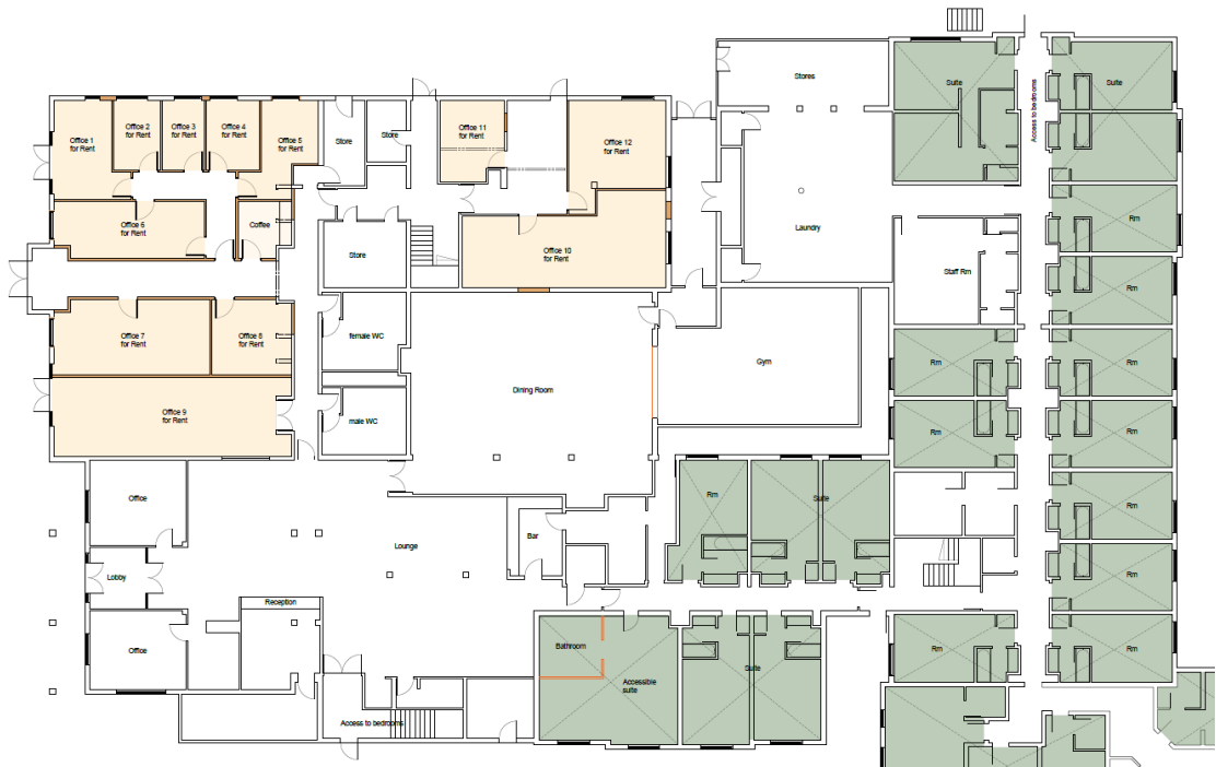
Above: Proposed Ground Floor Plan showing the proposed offices to rent
