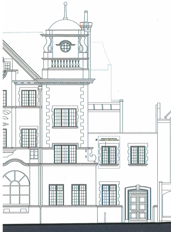
Existing window above entrance to residential development replaced
