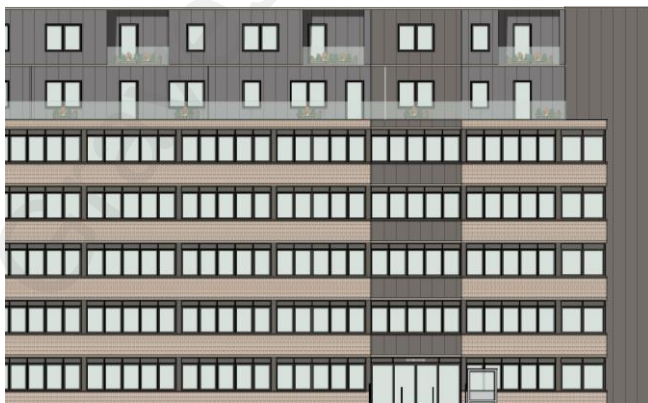
Part-elevation extract showing external alteration with proposed Class AA extension above (illustrative only)
