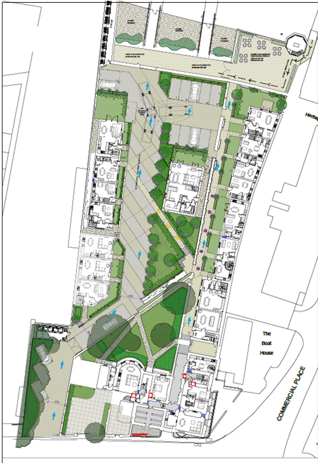
Figure 8.2 – Anticipated flow routes during an exceedance or blockage event.
