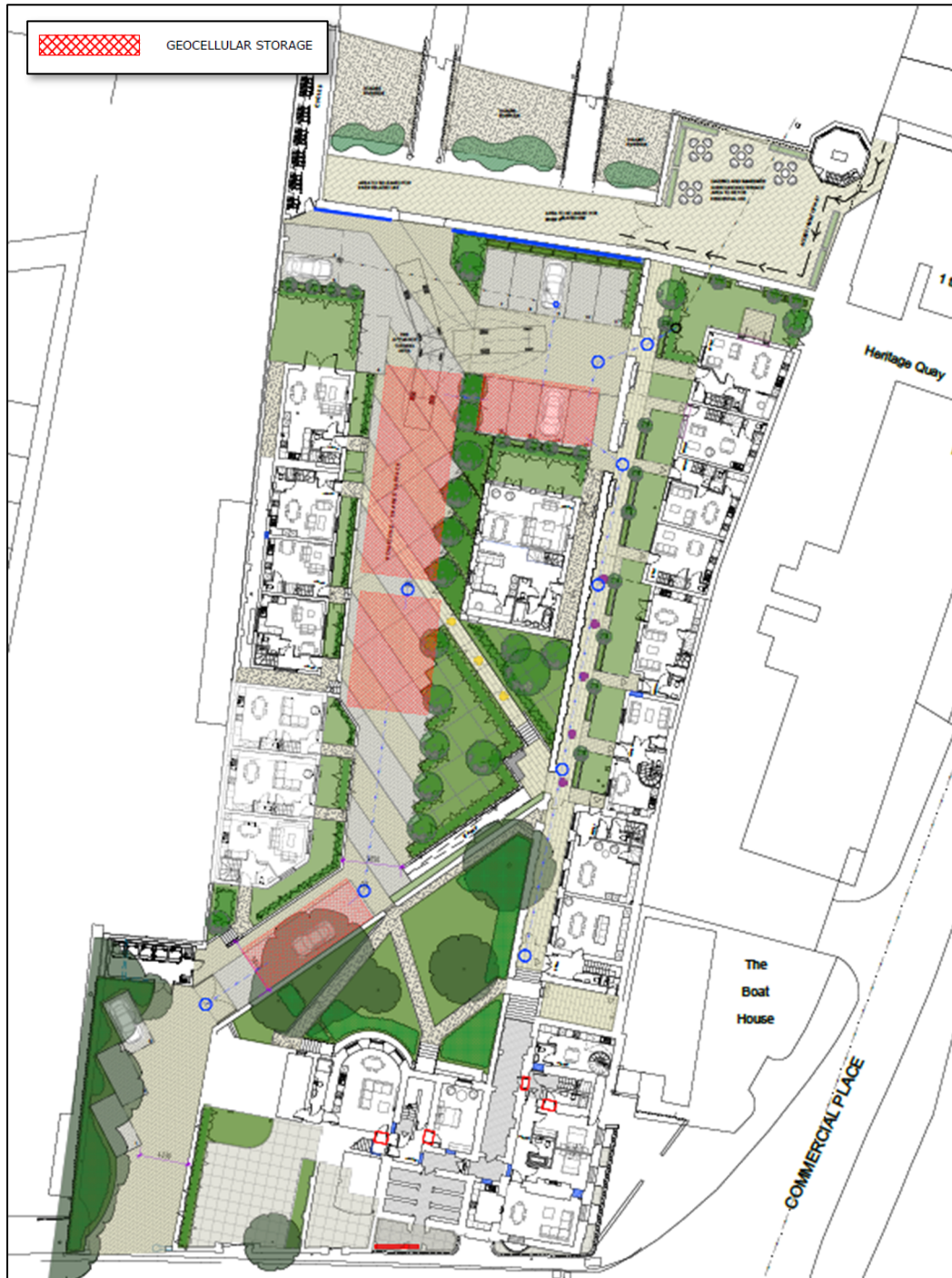
Figure 8.1 - Indicative drainage layout plan showing the proposed location of SuDS.
