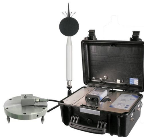
Fig. 12 Vibration Monitoring Equipment
