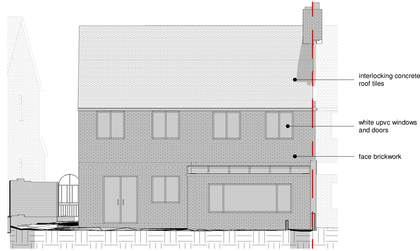
Rear Elevation / Existing
