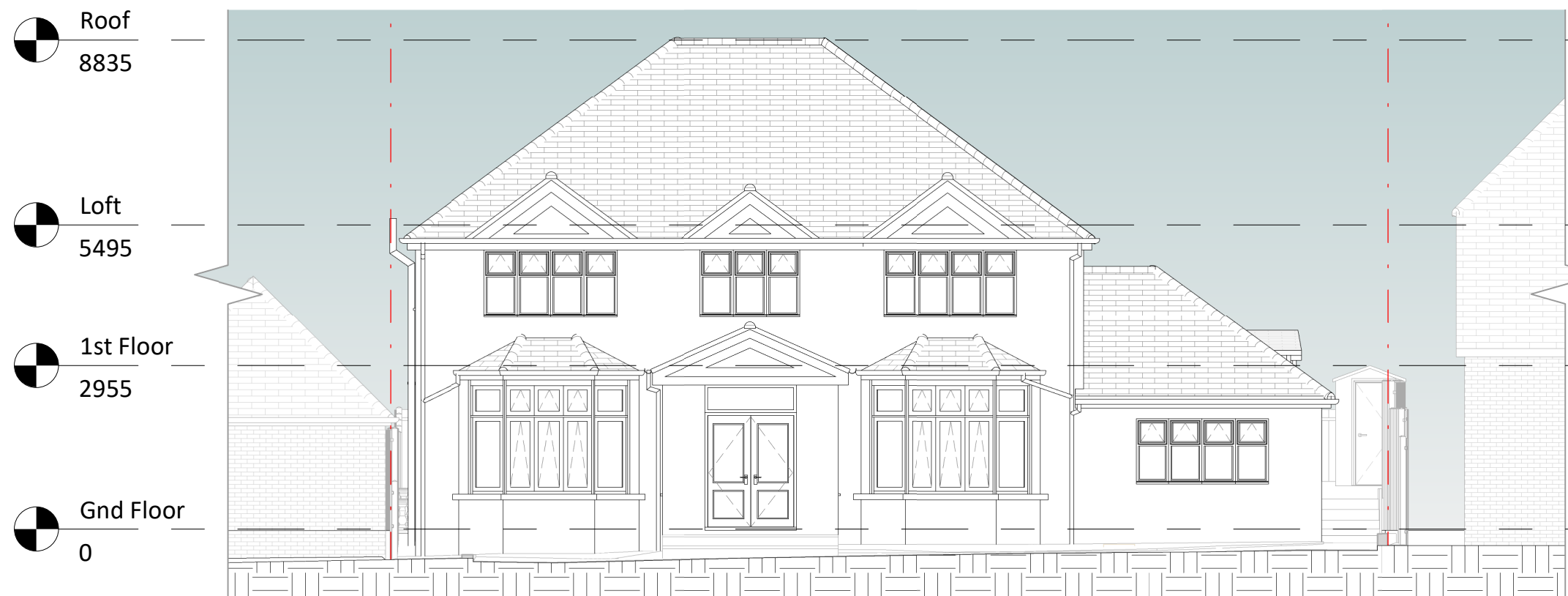
1 Existing West Elevation 1 : 100
