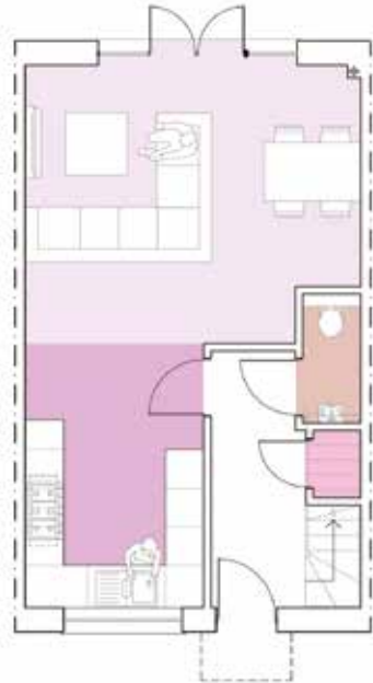
Typical 2 Bed Terrace Ground Floor
