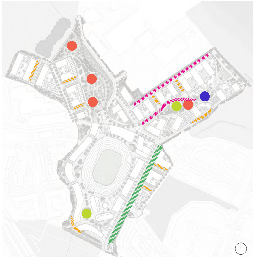
Illustrative Drainage and blue infrastructure treatment plan
