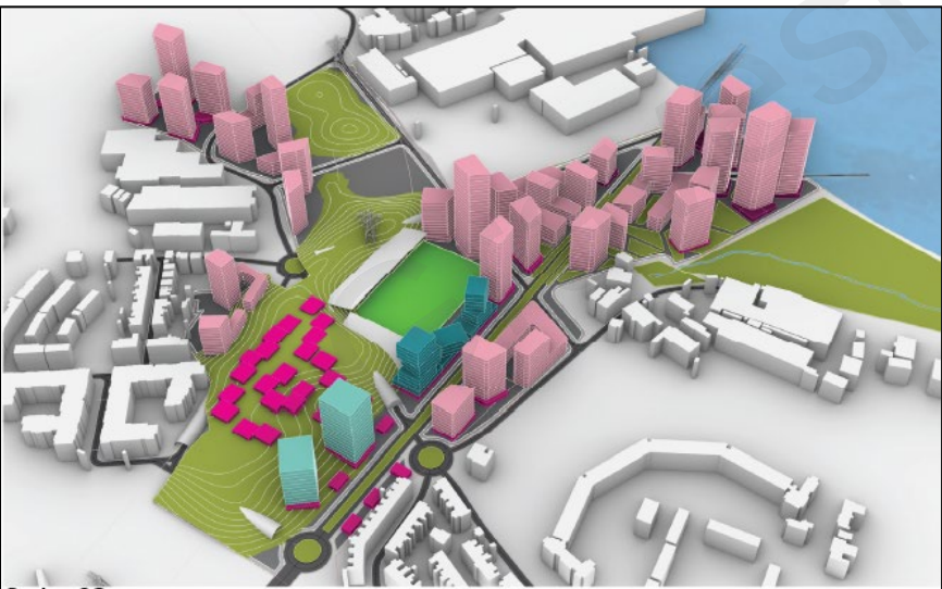
Option 2C. This option explores the placement of the South-East/ South-West connecting route as a dividing element between the retail village and stadium massing whilst still remaining under the terrain.
