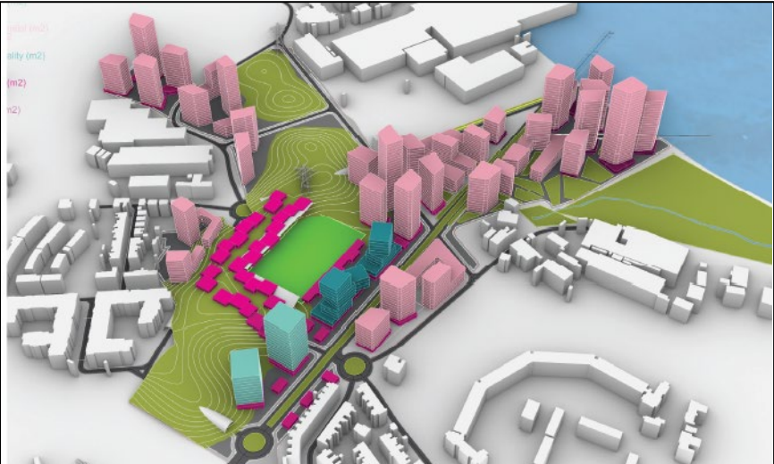
Option 2B. This option explores the placement of the South-East/ South-West connecting route centrally underneath the retail village adjacent to the stadium.
