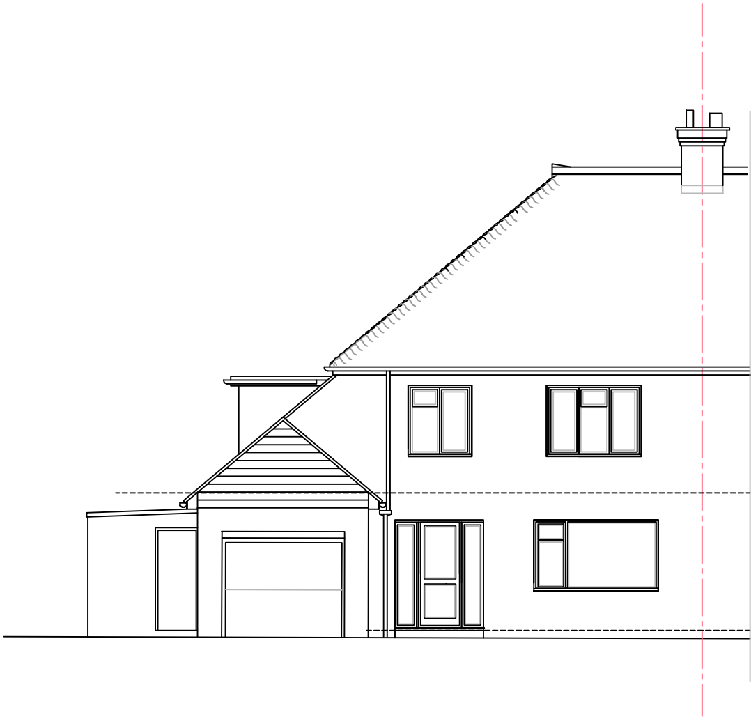
Existing Front Elevation (north east) Scale 1:100
